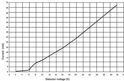
Fig. 3 Alarm load.
